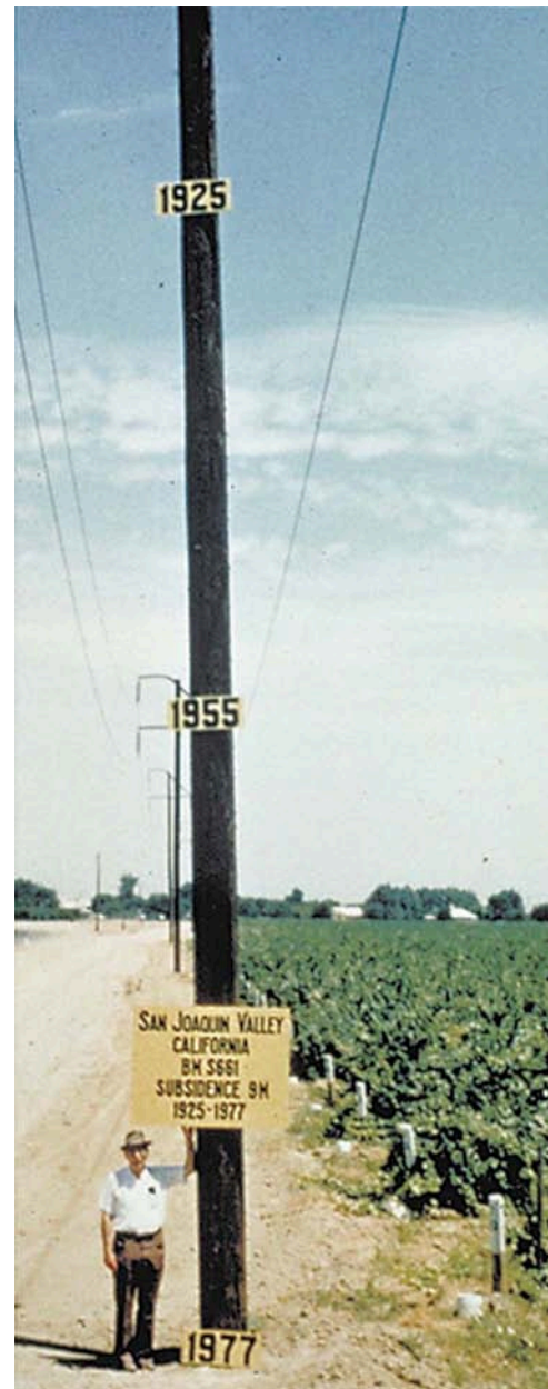
Figure 4-17. Illustration of maximum subsidence at a site 10 miles southwest of Mendota, showing 29.6 feet of subsidence between 1925 and 1977.
