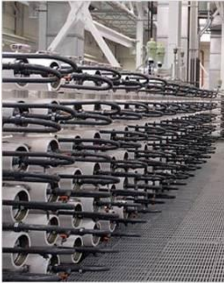
Reverse osmosis treatment is one step in the purification process that makes recycled water suitable for potable purposes
