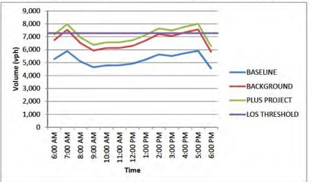
Segment ID Roadway From То SR 4 (Charter Way) CT 56 1-5 NB **Eighth St** 7,000 6,000 5,000 Volume (vph) Volume (vph) 4,000 BASELINE 3,000 BACKGROUND 2,000 PLUS PROJECT 1,000 LOS THRESHOLD 0 3:00 PM 7:00 AM 8:00 AM 9:00 AM 10:00 AM 11:00 AM 12:00 PM 1:00 PM 2:00 PM 4:00 PM 5:00 PM 6:00 PM 6:00 AM Time
