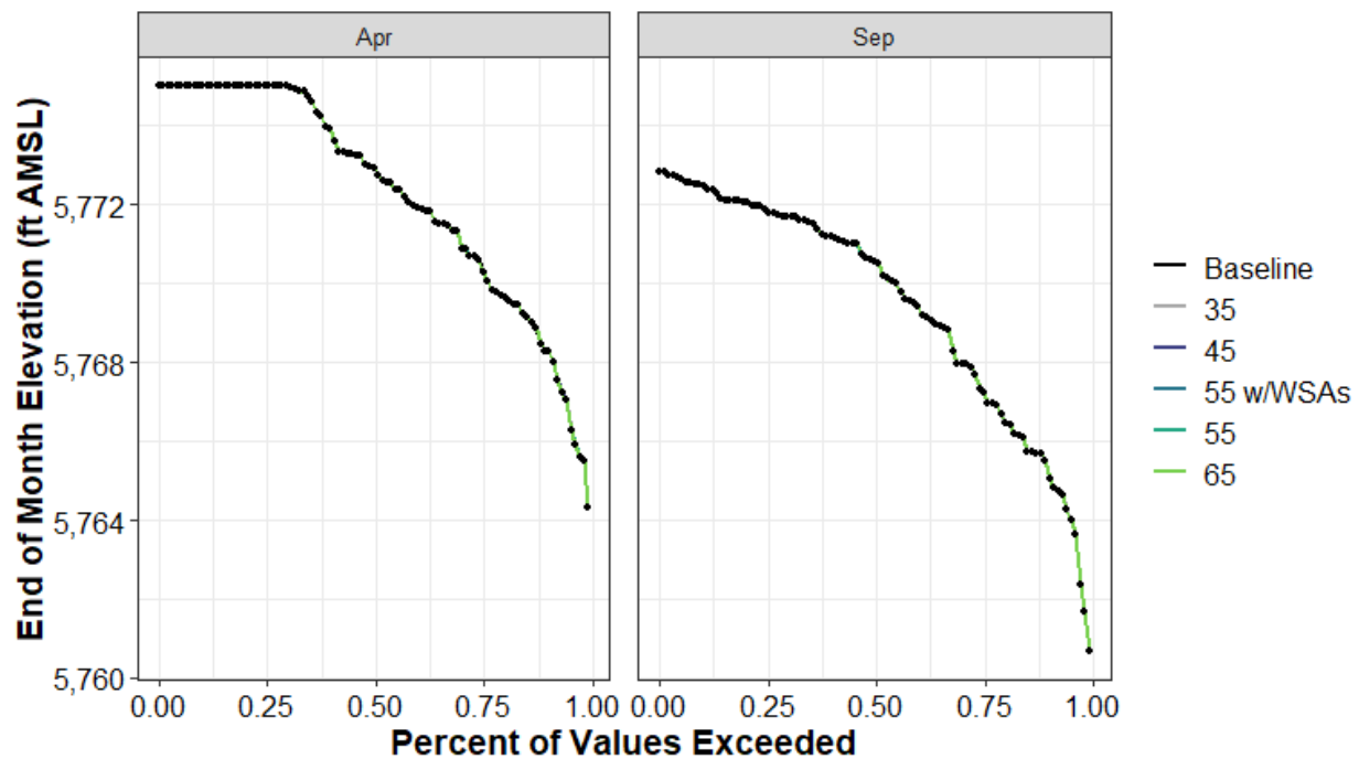
Figure H1a3-111. Lake Davis Reservoir End-of-April and End-of-September Elevation (ft AMSL) Percent Exceedance Plot
