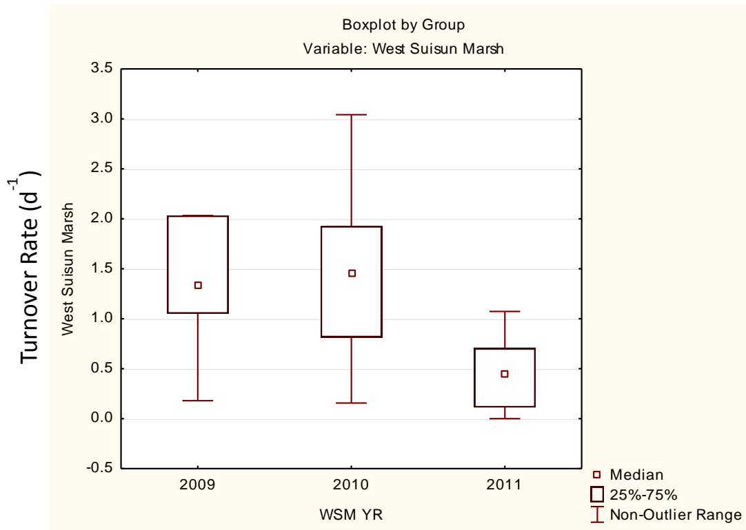
Figure 7b. Grazing rate normalized by water depth in West Suisun Marsh estimates water column turnover rate, the more conservative of the two calculated turnover rates.
