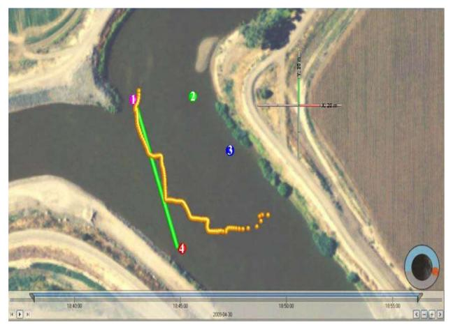
Figure 8-2. Acoustic tag tracking results for a juvenile Chinook salmon (yellow track) that was effectively guided downstream by the non-physical barrier (green line) at the Head of Old River (Source Bowen *et al.* 2009).
