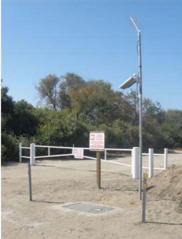
Well and data logger are below-ground in a vault (foreground). Power is supplied by a solar panel on the pole, and data are transmitted via satellite using the antenna on top of the pole.
