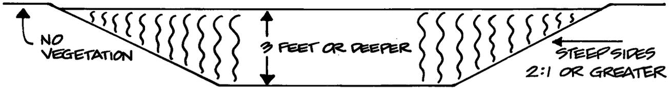
"STANDARD" EVAPORATION POND (2ppb TO 50ppb SELENIUM)
