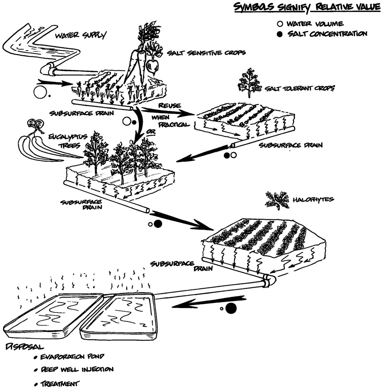
Figure 20. POND CONFIGURATIONS
