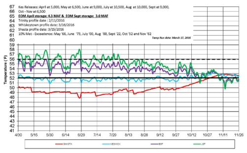
Figure 1. Reclamation's Sacramento River Water Quality Model (SRWQM) Temperature Results for May through November using the 2016 March 90% exceedance outlook, historical 10% local 3-month temperature outlook meteorology, Reclamation's proposed Keswick Dam monthly average releases, and targeting approximately 52°F DAT at KWK.
