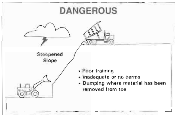
"Dangerous" stockpiling method (side view).
