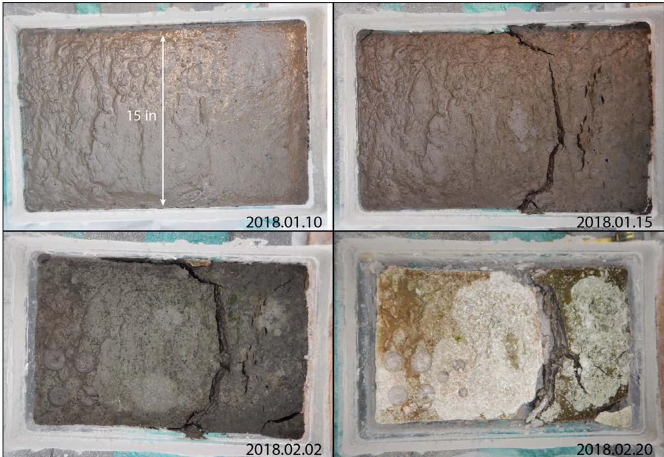
*Locations of Torvane measurements are visible on the left side of the February photos.*
